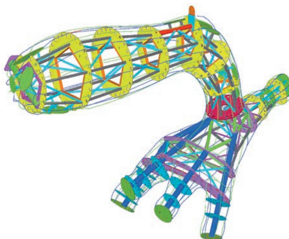
Obr. 4 – 3D model, jedna z nohou draka
